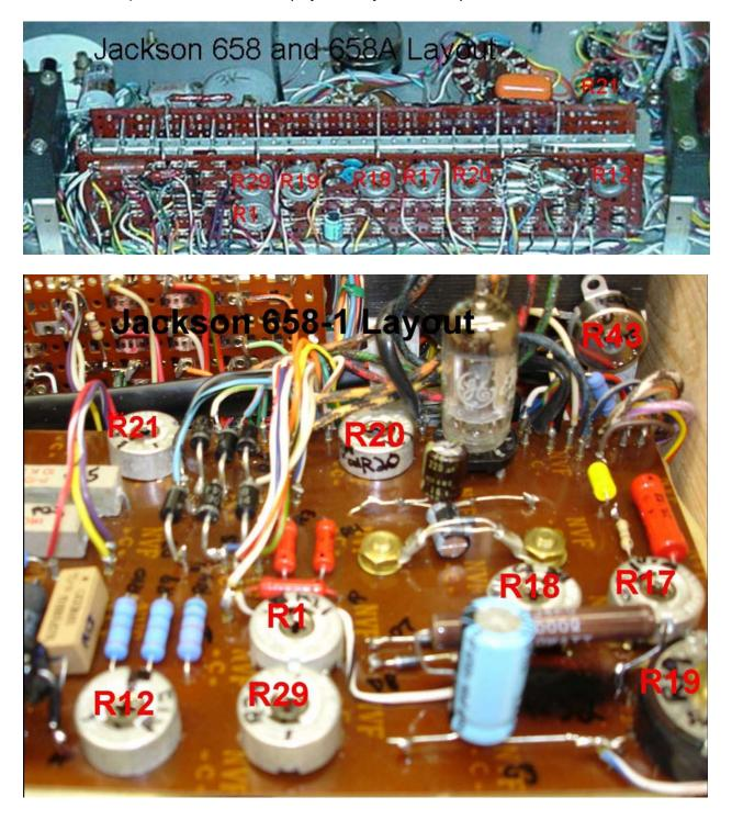
In all the procedures below, except as noted, set up the Jackson as if you're testing a 6L6 - 6.4L 123 top row 456 bottom row, 30Q, 45 for the grid control, and the rotary function switch set to "test." This setup will be used for all the following steps, which reference pins of the octal socket.
